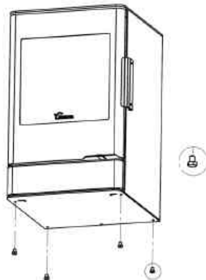
Figure No.15 - Installation of leveling feet
