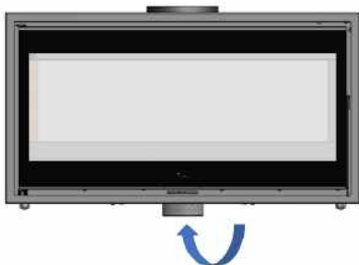
Figure No.10 - Conduction of the air intake for the combustion chamber
